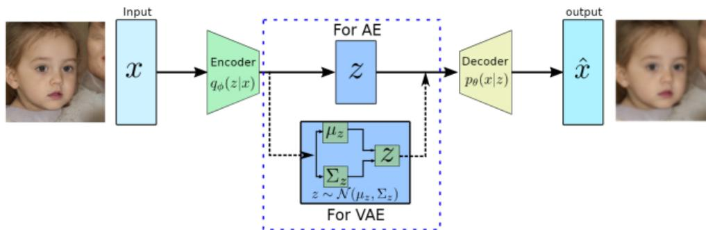
Figure: AE vs. VAE architecture
