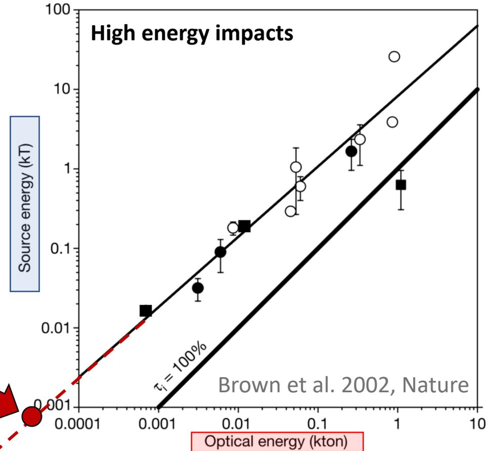
**Figure 2** Bolide energy calibrations. These are based on simultaneous observations by optical sensors (or equivalent) and energy estimated from another technique. The optical
