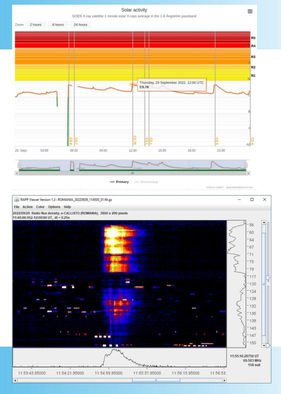
After installing the new front end we record two radio burst in the same day, 11.10.2022.
