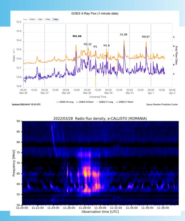
In the bottom picture is a Type V radio burst recorded in 29 september 2022 at 11.54 UTC with a duration of 5 minutes. It follows a C5.76 flare in AR 13112.
