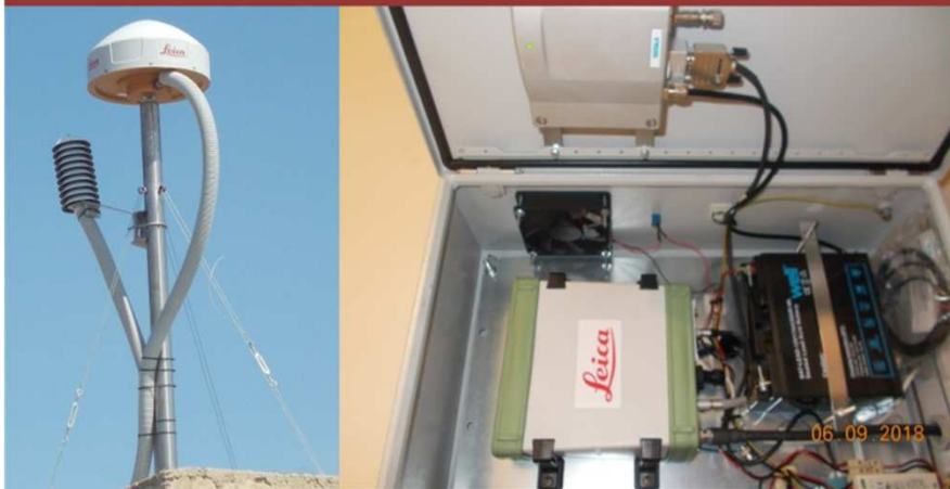
GNSS REFERENCE STATION & METEOROLOGICAL STATION - KLIR
